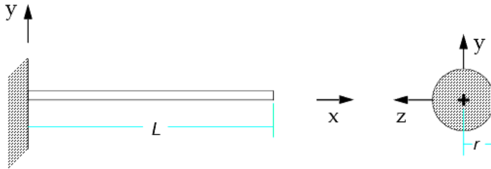
Figure 4-8. Cantilever Beam Model
