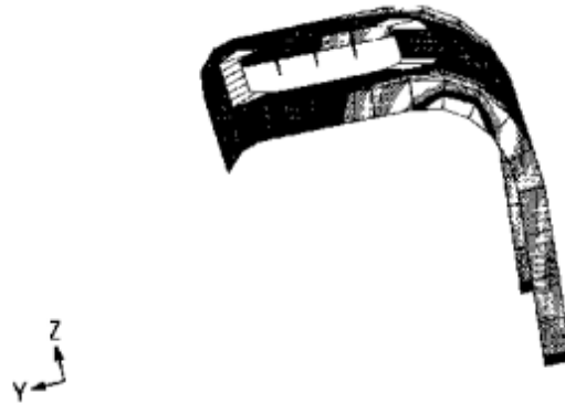
Figure 4-19. Element Strain Energy Contours for the Third Mode
