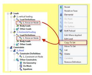
Figure 15: The Move and Copy To Set commands in typical usage.
