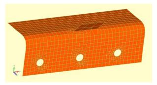
Figure 11: Surfaces meshed and new features embodied into flange model.
